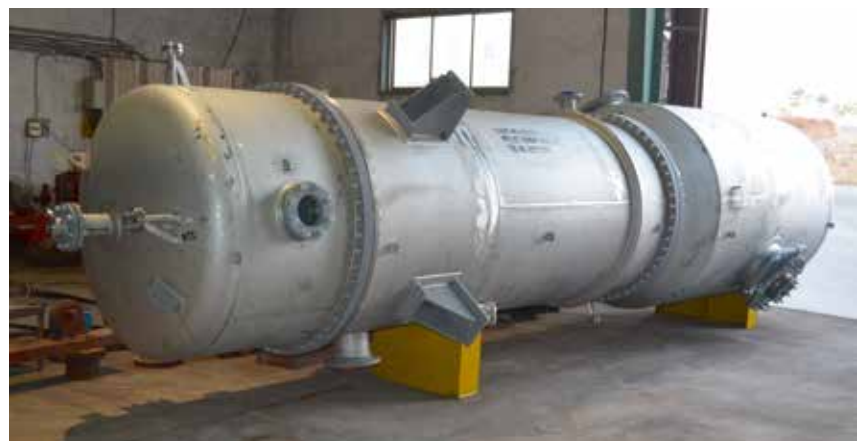
⌚ Falling film evaporator exported to Malaysia (DOSH compliant).
