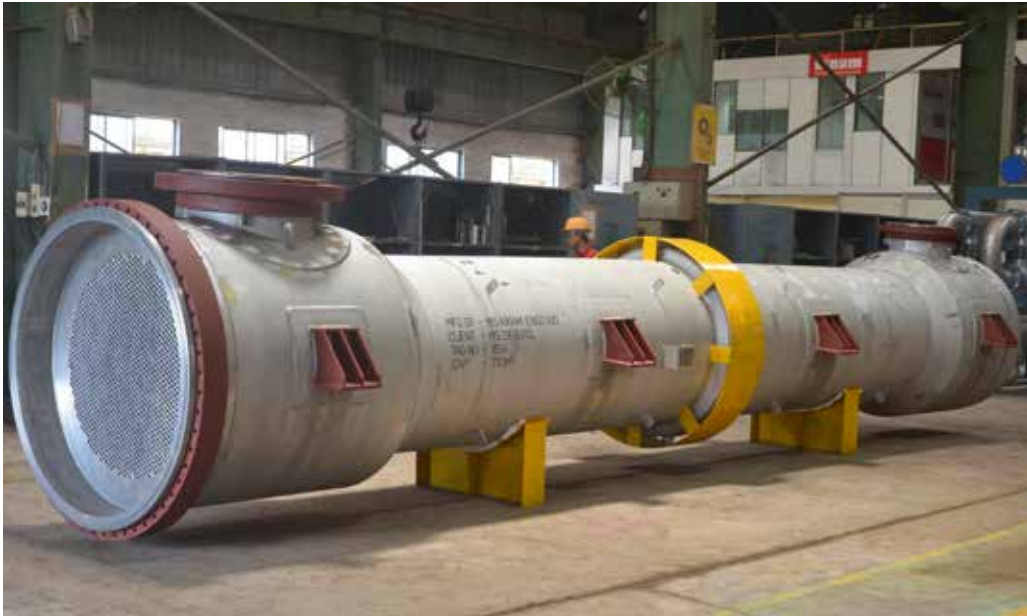
⌘ Fixed tubesheet type-710 m 2 tail gas heater.
