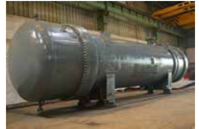
⌘ Floating head type 1458 m 2 depropanizer condenser (4032 tubes).
