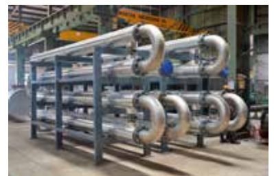
⌘ Double pipe type Sludge heater for a sewerage treatment plant.
