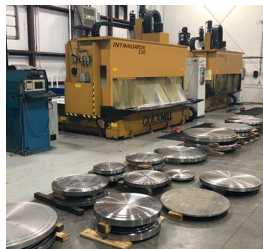
➤ A selection of Ward Vessel & Exchanger tubesheets in the company's new machine shop.
