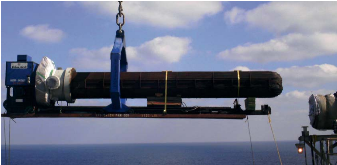
« Aerial hydraulic exchanger bundle extractor.
