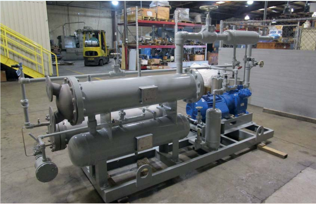
« Refrigerated sea water skid package for a small boat in Pakistan
