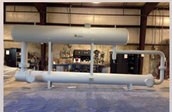
⚡ R-507a-glycol thermosyphon evaporator for petrochemical
