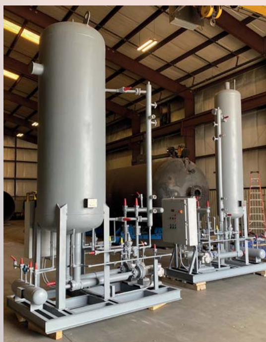
Ammonia liquid recirculator skid packages for solid storage
