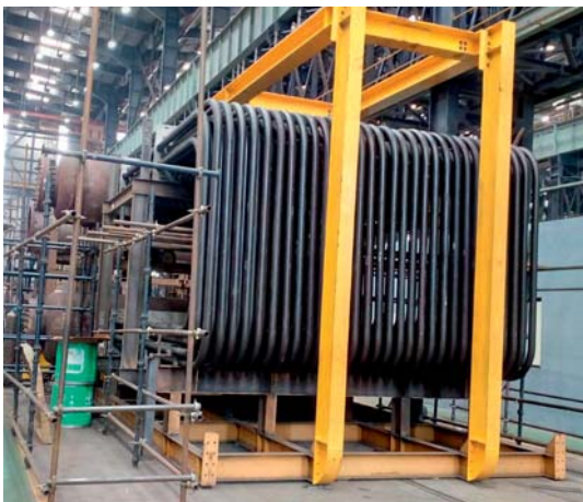
➤ Special shape critical U-tubes of T11 grade (88.9 mm x 4 mm) WT x 15 meters in length.
