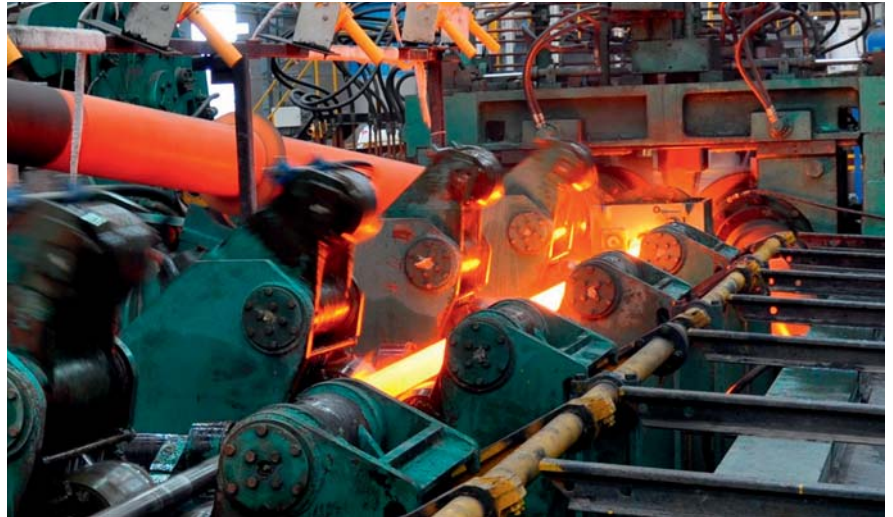
➤ One of the factors that separates it from the competition is Heavy Metal & Tubes' ability to produce its own mother hollows in stainless, carbon, and alloy steel. Shown here – the production of mother hollows from round bar.
