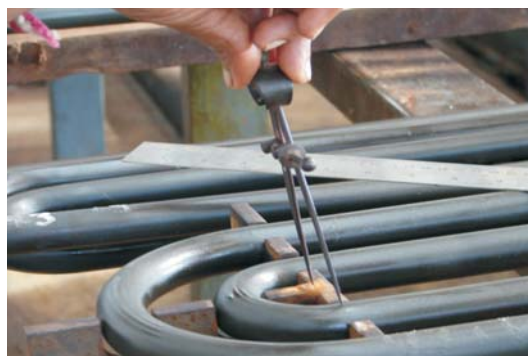
➤ The accuracy of the U-bend tubes is ensured by precisely prepared jigs and fixtures.
