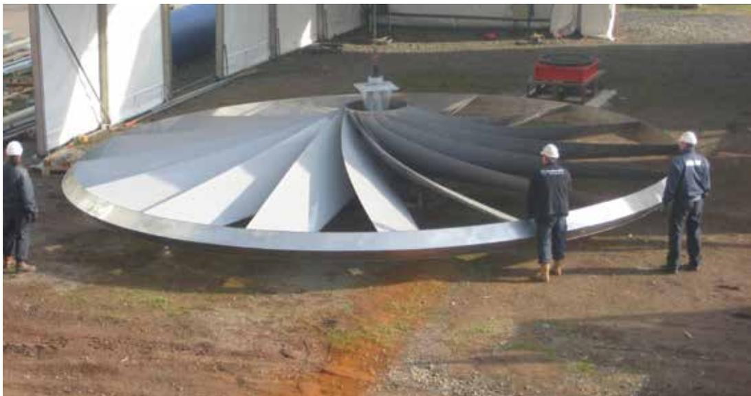
We ourselves designed a fan system and we can use this in newly or retrofitted air-cooled heat exchangers. It is so called the Whizz-Wheel®."
