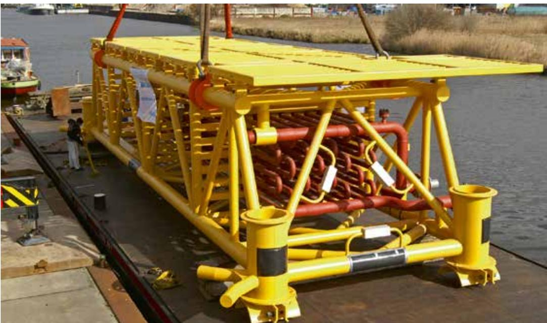
« Bronswerk Heat Transfer is one of the few companies in the world capable of designing and manufacturing subsea coolers.
