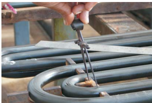
➤ The accuracy of the U-bend in tubes is ensured by precisely prepared jigs and fixtures.
