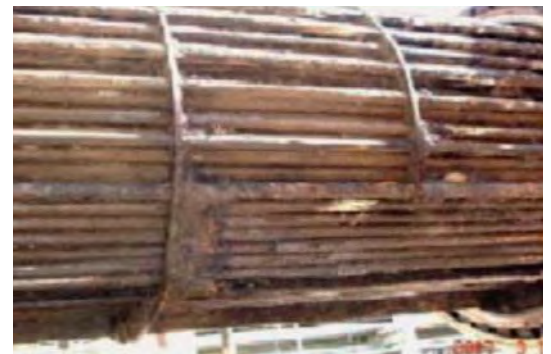
Bundle with cooling water in shell side.
