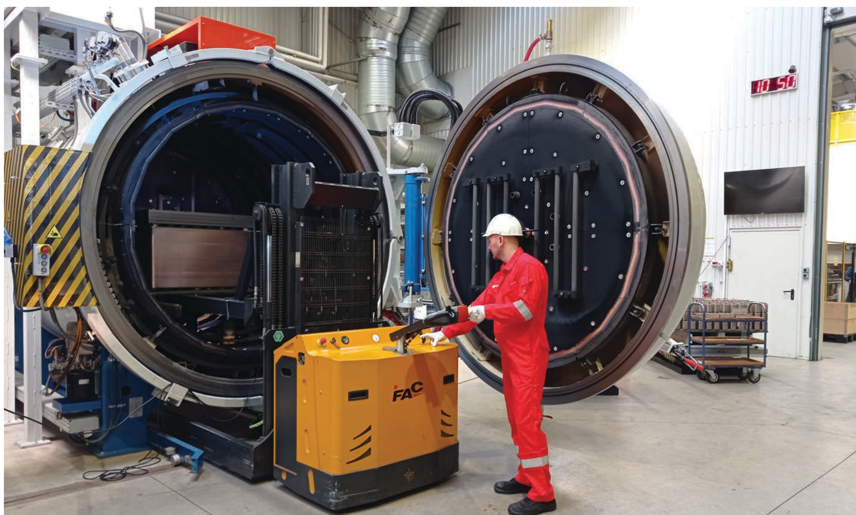
➤ Brazed plate heat exchanger LE400 brazed in vacuum furnace. Soon to be installed in a heat substation of a furniture factory in Poland. Hexonic BPHEs enable high thermal performance at low operating costs.
