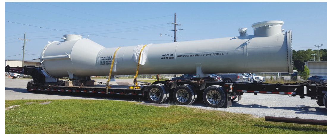
» Shipment of a sulphur condenser exchanger with an empty weight of 112,900 pounds.
