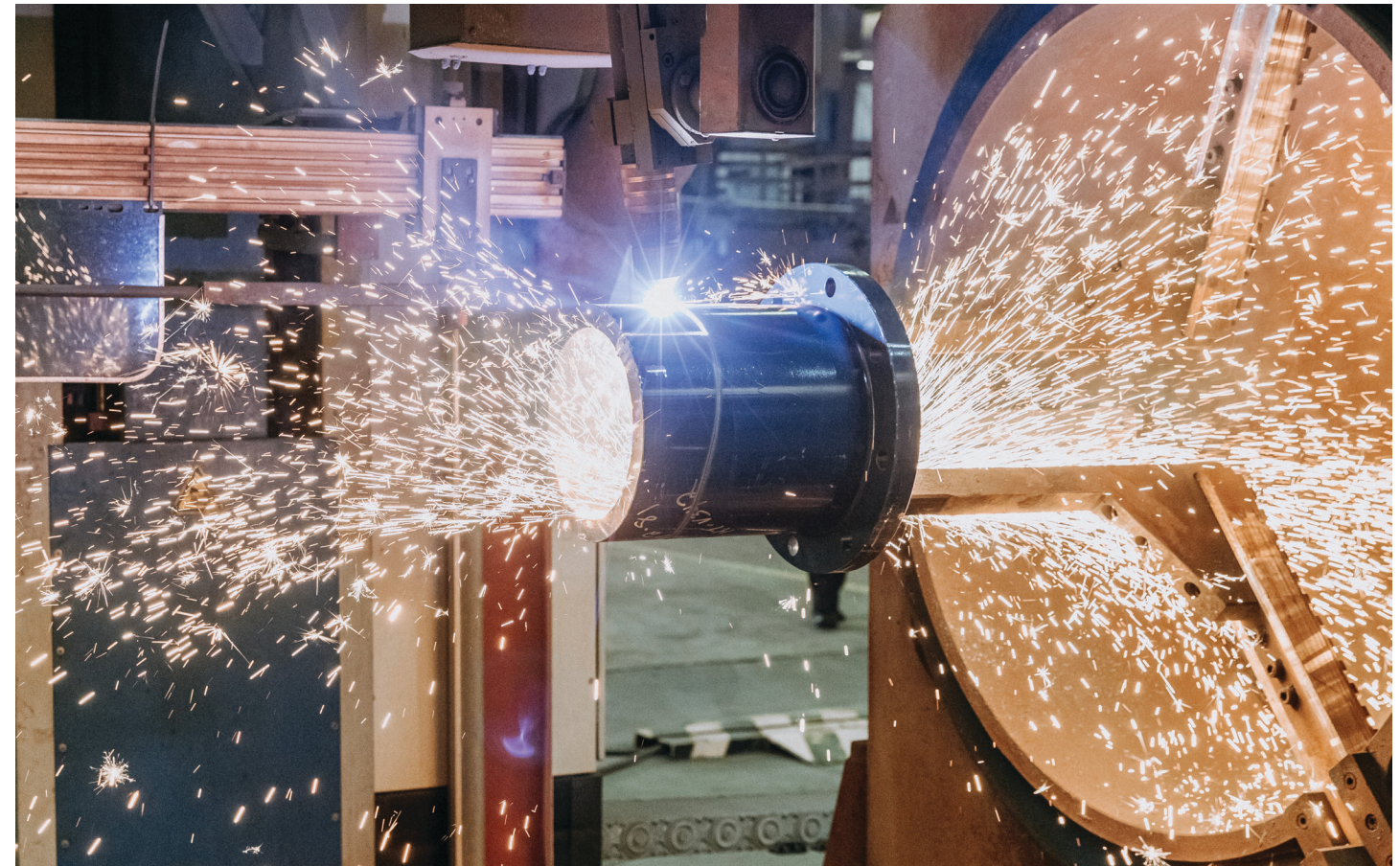
» CNC automated profiling of a nozzle using a multi-axis head machine.
