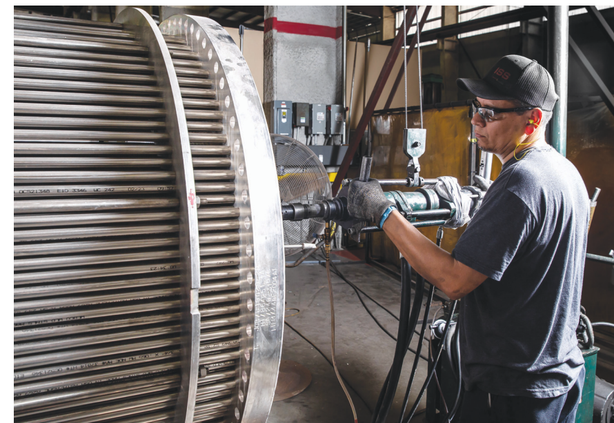
➤ Tube rolling using parallel pin expansion.
