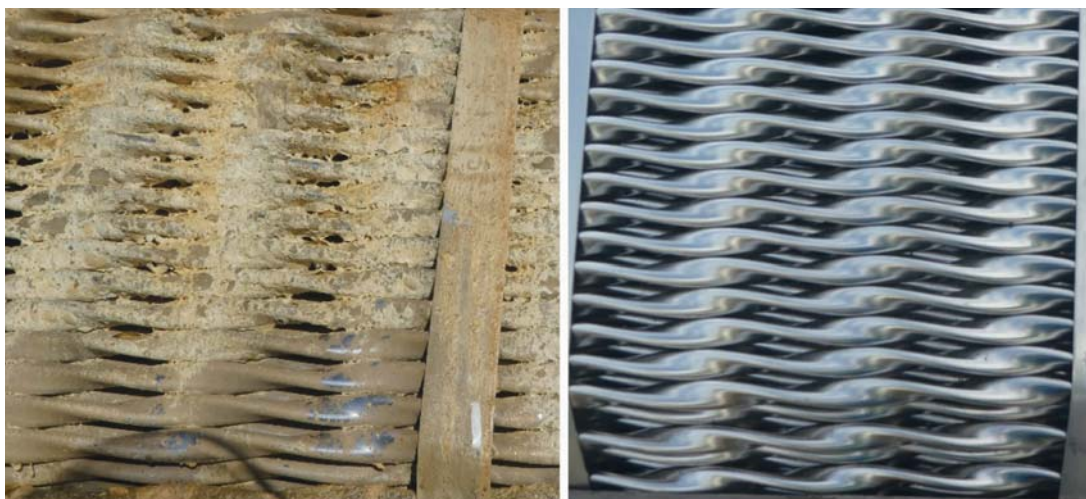
➤ Figure 3. Twisted Tube® bundles cleaned using ultrasonic technology (courtesy TechSonic)
