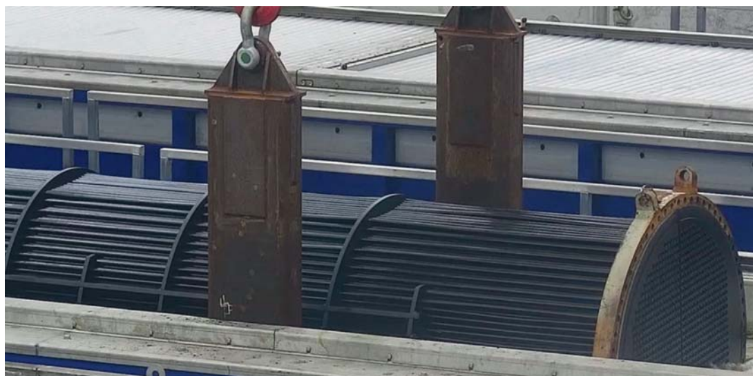
Figure 1. A heat exchanger being lowered into an ultrasonic bath (image courtesy of Clean As New)
