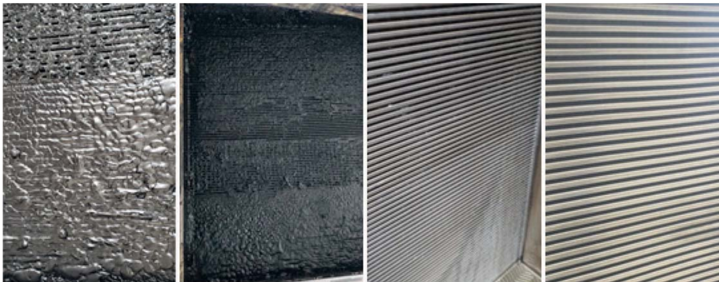
➤ Figure 2. A badly fouled welded plate exchanger, cleaned using ultrasonics.
