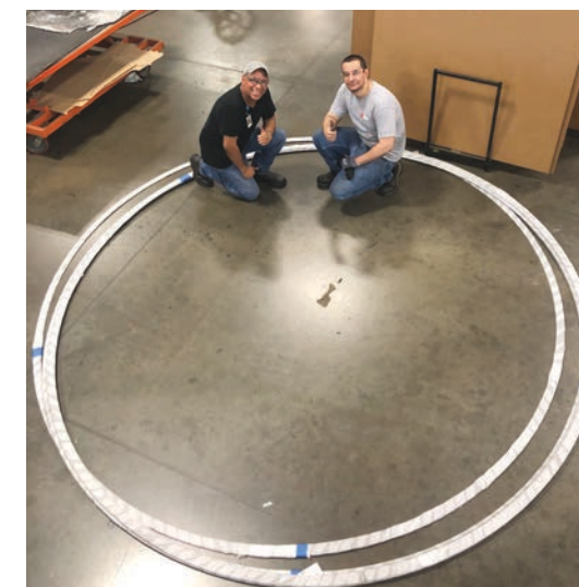
TEADIT is often sought out for its ability to be able to handle heat exchanger projects requiring over sized Camprofile Gaskets.
