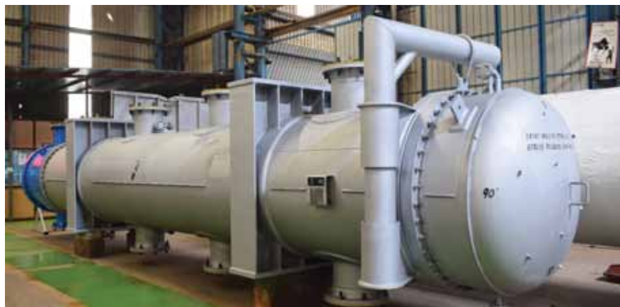
Figure 3. Removable tube bundle heat exchanger.
