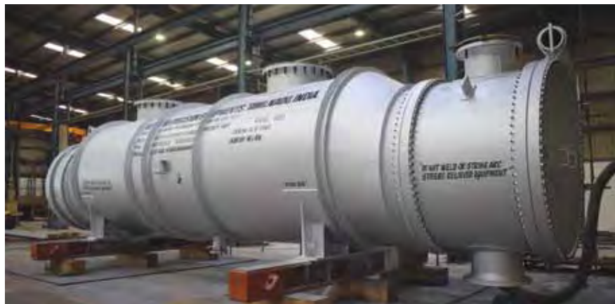
Figure 2. Kettle type heat exchanger with fixed tube bundle.
