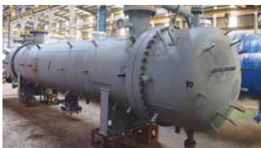
Figure 5. Floating head type heat exchanger.
