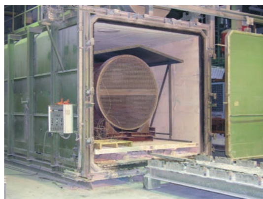
➤ Thermo-Clean's specially developed pyrolysis ovens give the team a high level of oxygen and temperature control meaning they can accurately monitor what happens during the gasification of organic fouling.
