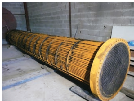
➤ Shell and tube heat exchanger on the left was pre-cleaned with high-pressure and declared clean by the customer. Yet after thermal cleaning (photo on the right), we removed additional 200 kilos of fouling.
