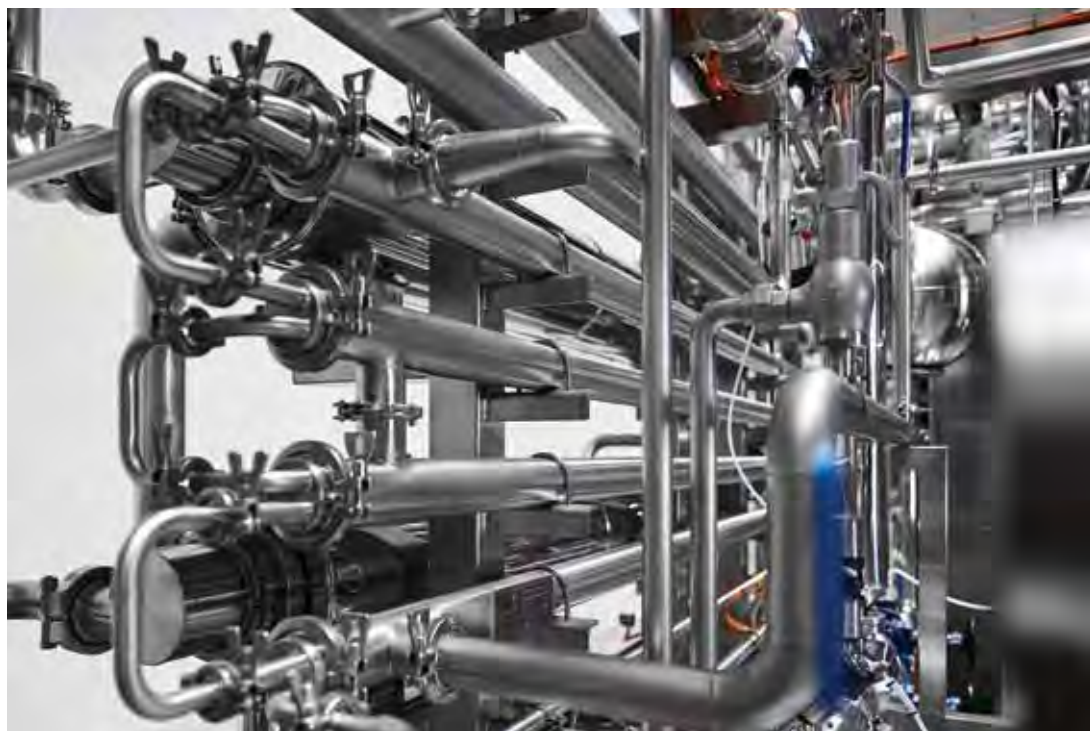
⚡ MI Series heat exchangers are often combined with scraped surface units such as the R Series.
