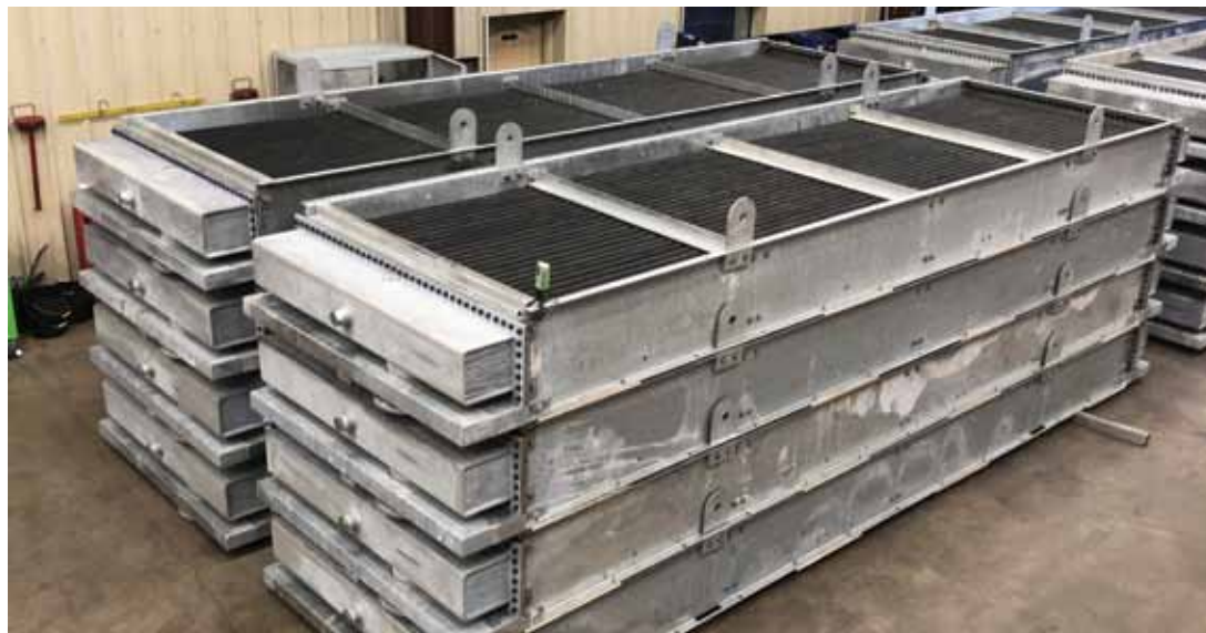
Figure 3. Plume abatement coil
