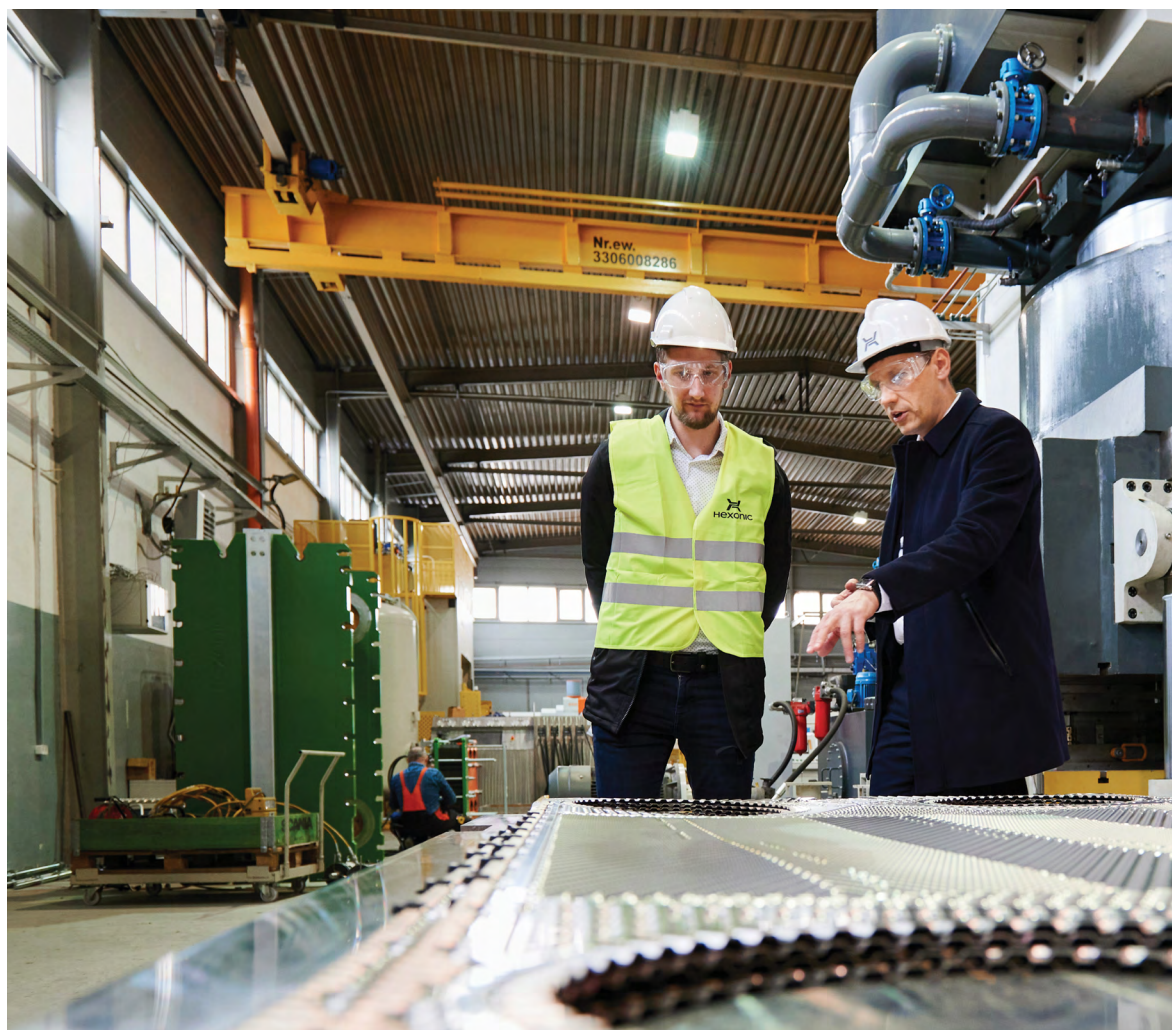
↗ Hexonic's JAG plate design features a unique corrugated pattern to increase heat transfer efficiency.
