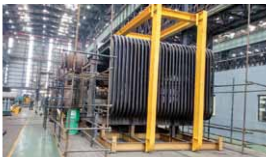
Special shape critical U-tubes of T11 grade (88.9 mm x 4 mm) WT x 15 meters in length.
