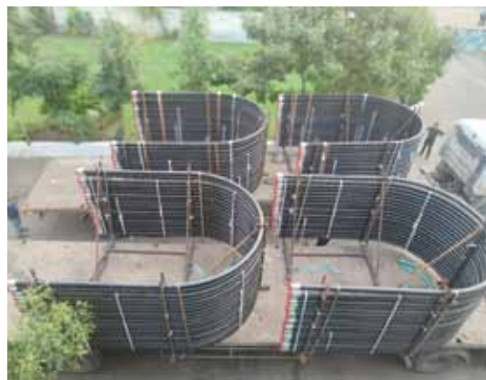
➤ Heavy Metal has successfully manufactured arbor coil bends for the first time in India.
