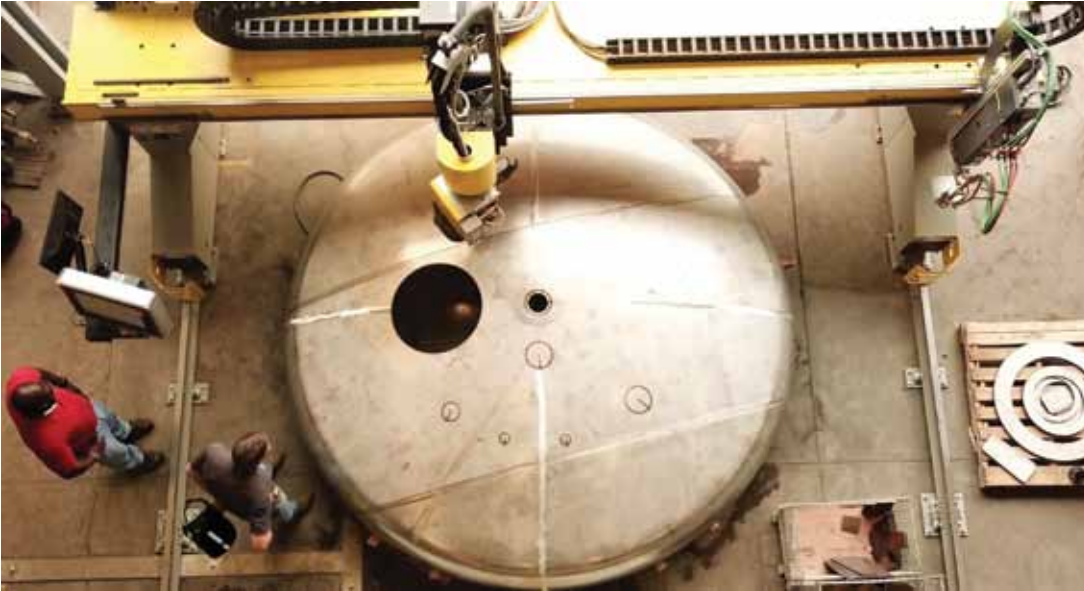
↻ 5-axis burn table technology laying out and cutting nozzle penetrations in the dished head.
