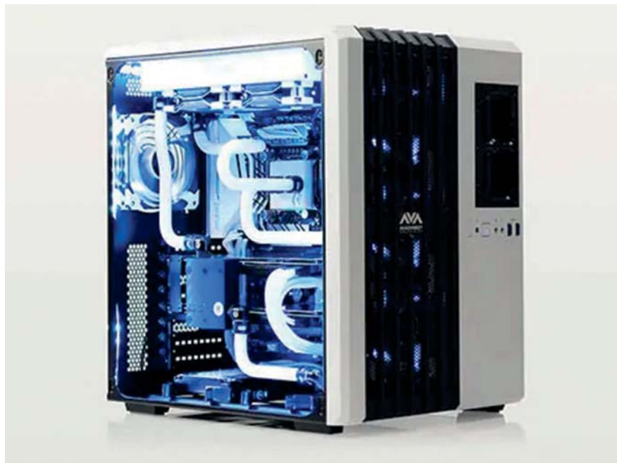
⚡ Electronic components are typically air-cooled with a fan and a heat sink, but for hotter applications, such as gaming PCs and electric powertrains, indirect liquid cooling is used. Image courtesy of Avadirect.
