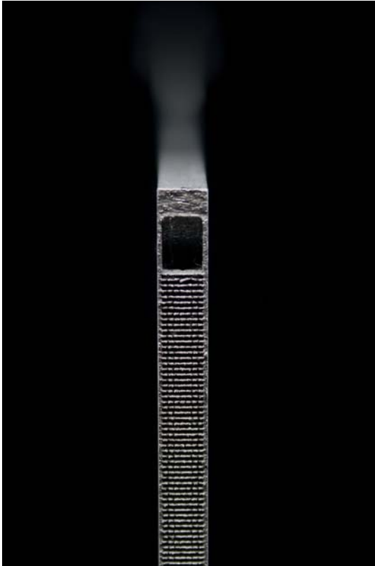
✦ Conflux Technology creates advanced additive manufactured cold plates for electronics and battery cooling. Additive manufacturing allows complex internal geometries which help direct and mix the flow as well as increase surface area.
