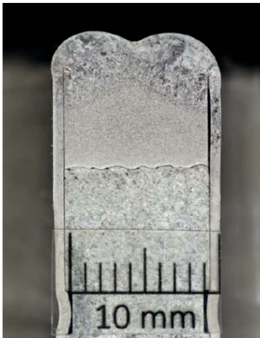
⚡ Macro examination with 3.5% magnification of cladded tubesheet.
