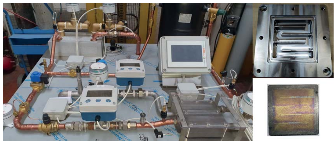
➤ The image on the left is the experimental setup. The test rig is fitted with temperature, flow, and pressure sensors and the data was used to calculate the heat transfer coefficient of tested materials. On the right side is the heat exchanger where a plate is placed into the slot as shown. During the test, a working fluid flows on one side and a geothermal brine on the other side.
