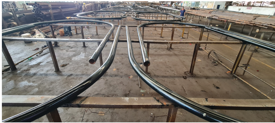
Heavy Metal has successfully manufactured arbor coil bends for the first time in India.
